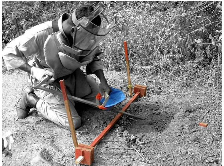
The photograph shows a deminer in Sri Lanka using the SD Two-handed excavator. In the very hard ground, he is digging well back from the red detector signal marker and can do so quickly and easily.
